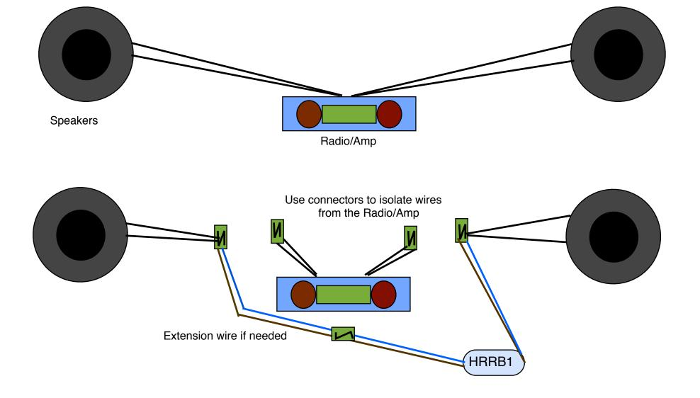
If the music breaks up at the highest volume it may be due to your speakers being lower than  $3\Omega$  If this is the case please get in touch and we will send out two wired resistors, they just clip into the existing set up, this should resolve the problem.
